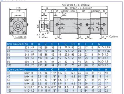
Remark: The dimensions of magnet type cylinder are the same as non-magnet type cylinder
