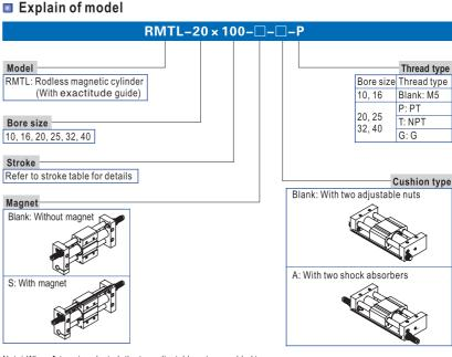
Note) When  ${\bf A}$  type is selected, the two adjustable nuts are added too.
